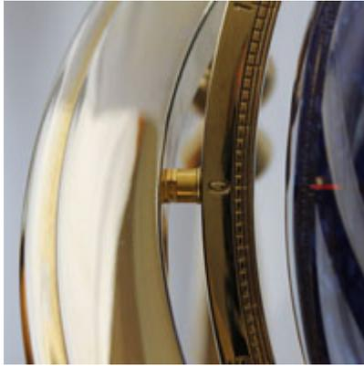
The cure for your sagging globe is to increase the friction in the mount between the meridian ring to the horizon ring. With a little bit of instruction, a person possessing reasonable mechanical aptitude can expect to make the necessary adjustment and restore the globe to its original condition.
